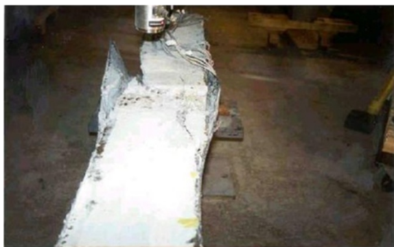
Figure 18 Failure of Beam-0°/90°/45°.
