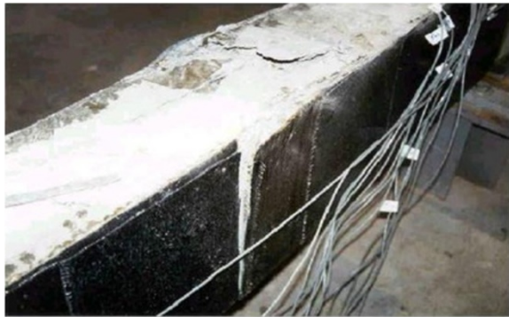
Figure 17 Failure of Beam-0°/90°.
