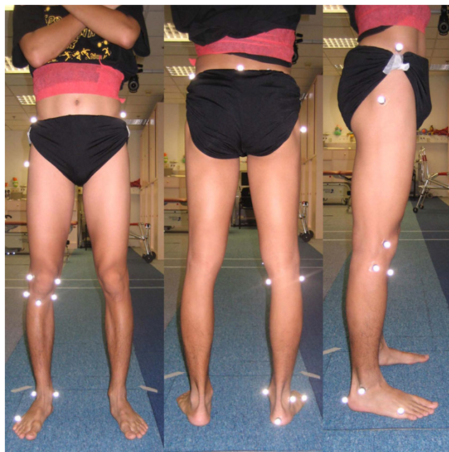
Figure 9 Marker set of motion analysis assessment (Left to right: anterior view, posterior view and lateral view).
