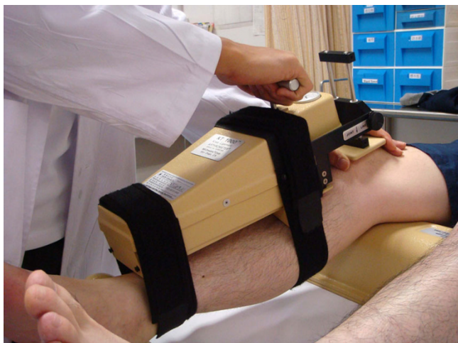
Figure 5 KT 1000 to measure anterior-posterior laxity of the knee.
