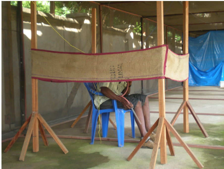
Figure 1 Transfluthrin hessian strip. The hessian strip is made from fine sisal fiber woven together to make sacking fabric. The strip is 4 × 0.3 m long. It is treated with transfluthrin. The strip is suspended on 4 wooden poles making approximately 1 m 2 area surrounding the human participant conducting mosquito catches.
