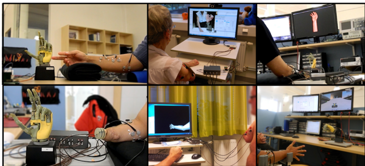
Figure 16 Non-amputee and amputee subjects demonstrating BioPatRec applications. The different insets in this figure show amputees and non-amputees using BioPatRec for the control of a multifunctional prosthesis; virtual limbs in augmented and virtual reality; and computer games. All these potential output possibilities from BioPatRec as a motion predicting software.
