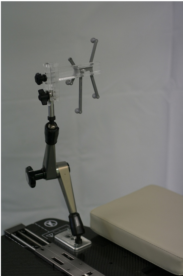
Figure 2 Infrared-Mechanical Arm unit. An infrared reference frame is connected to the mechanical arm which in turn is connected to the treatment table via a self-centering bracket. Before patient positioning, the arm and IR-frame are rotated out of the way as shown so the patient can lie down on the headrest.
