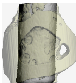
Figure 3 3a and 3b. 3-D microCT view of a titanium implant (a) and illustration of defined peri-implant VOIs (b.)
