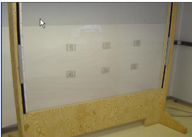
Figure 3 Physical target grid for virtual environment calibration.
