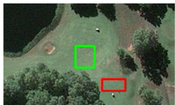
Figure 8 Another tailored remote sensing image. The two regions specified by red and green rectangles are homogenous regions. They are used to compare texture describing ability of RIU-LBP and improved RIU-LBP.
