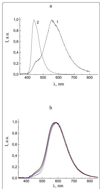
**Figure 3 Normalized EL spectrum of devices 6 and 7. (a)** Normalized EL spectrum of device 6, ITO/PTA/NPD/Zn(TSA-BTZ)<sub>2</sub>/Al: Ca, (1) and PL spectrum of Zn(TSA-BTZ)<sub>2</sub> powder (2). **(b)** Normalized EL spectra of device 7, ITO/PTA/Zn(TSA-BTZ)<sub>2</sub>/Al:Ca, for bias voltages 3.5 (blue curve), 4.0, 4.5, 5.0, 5.5 (black curves), and 6.0 V (red curve).
