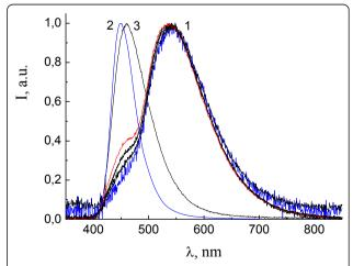
**Figure 4 Normalized EL spectra of device 8, ITO/PTA/NPD/Zn (POPS-BTZ)<sub>2</sub>/Al:Ca.** For bias voltages 4.0 (blue curve), 4.5, 5.0, 5.5 (black curves), and 6.0 V (red curve) (1). PL of Zn(POPS-BTZ)<sub>2</sub> powder (2), and the EL spectrum of device 9, ITO/PTA/NPD/CBP/Zn (POPS-BTZ)<sub>2</sub>/Al:Ca, (3).
