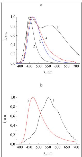
**Figure 2** EL spectra of Zn(PSA-BTZ)<sub>2</sub> in devices 1 and 2. (a) EL spectrum of device 1, ITO/PTA/NPD/Zn(PSA-BTZ)<sub>2</sub>/Al:Ca (1); PL spectrum of Zn(PSA-BTZ)<sub>2</sub> powder (2); EL spectrum of device 3, ITO/PTA/NPD/CBP/Zn(PSA-BTZ)<sub>2</sub>/Al:Ca (3); and EL spectrum of device 5, ITO/PEDOT:PSS/Zn(PSA-BTZ)<sub>2</sub>/Al:Ca (4); **(b)** EL spectra of device 2, ITO/PTA/Zn(PSA-BTZ)<sub>2</sub>/Al:Ca, (1) and device 4, ITO/PTA/CBP/Zn(PSA-BTZ)<sub>2</sub>/Al:Ca (2).
