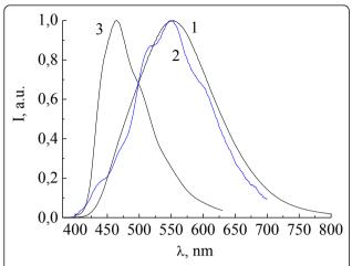
Figure 5 EL spectra of devices 10, ITO/PTA/NPD/Zn(DFP-SAMQ) <sub>2</sub>/Al:Ca, (1) and 11, ITO/PTA/Zn(DFP-SAMQ)<sub>2</sub>/Al:Ca, (2). PL of Zn (DFP-SAMQ)<sub>2</sub> powder (3).
