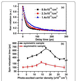
Figure 4 Photo-excited carrier density dependence of electron spin relaxation times measured at 10 K with excitation wavelength of 798 nm. (a) The typical time-resolved Kerr rotation signals measured at three different pumping electron densities for the asymmetric GaAs QW. (b) Photo-excited carrier density dependence of electron spin relaxation times measured for both symmetric and asymmetric GaAs QW samples. The solid lines are drawn to guide eyes.
