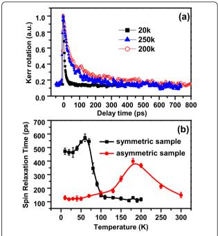
Figure 3 Temperature dependence of electron spin relaxation times measured at excitation wavelength of 798 nm and optically pumped electron densities of  $1.15 \times 10^{11} \text{ cm}^{-2}$ . (a) The time-resolved Kerr rotation signals measured at 20, 200, and 250 K for the asymmetric GaAs QW. (b) Temperature dependence of electron spin relaxation times measured for both symmetric and asymmetric GaAs QW samples. The solid lines are drawn to guide eyes.
