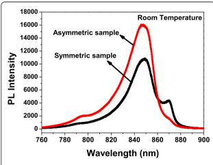
Figure 2 The PL response measured at room temperature for both symmetric and asymmetric GaAs/AlGaAs QWs.
