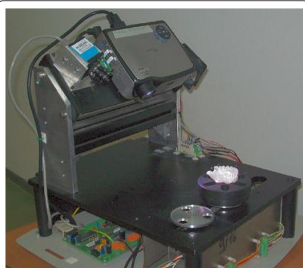
Figure 1 Optical scanner. 3D optical scanner used to capture dental models.
