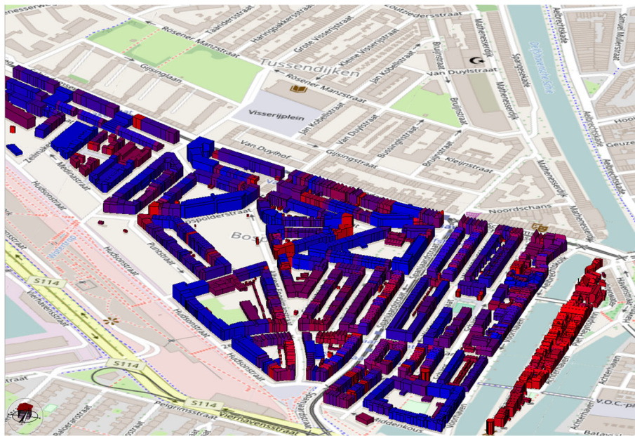
Fig. 17 CityGML model of Rotterdam: Visualisation of the simulated annual heating energy demand per square meter of floor area
