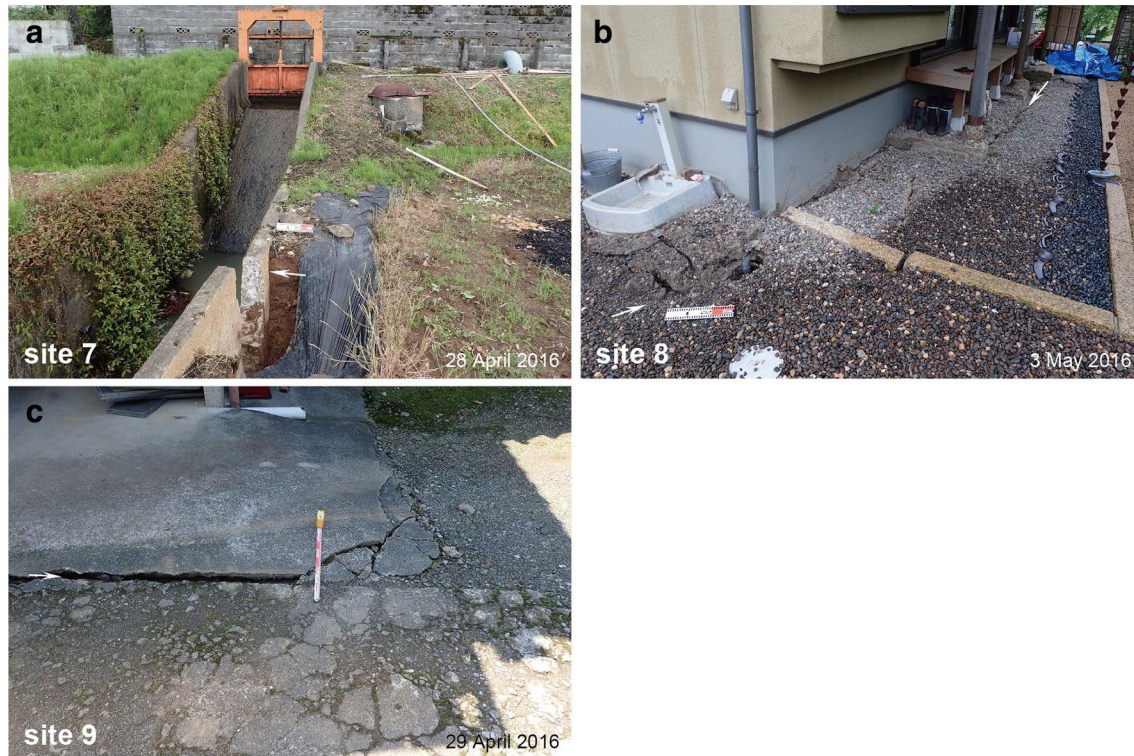
Fig. 5 Snapshots of surface ruptures related to the largest foreshock and mainshock at each site shown in Fig. 1. a Right-lateral offset of a creek. The dextral offset was ca. 20 cm after the mainshock, almost half of which was associated with the largest foreshock. b An open crack, which appeared in association with the largest foreshock and later enlarged due to the mainshock. c An open crack, whose width was ca. 2 cm after the largest foreshock and ca. 5 cm after the mainshock
