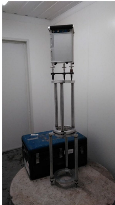
Fig. 15 Measuring setup at Peistareykir for determination of the free-air vertical gravity gradient with the help of a CG5 Scintrex gravity meter and a tripod; gravity measurements were performed directly on the concrete pillar, at 60 cm and at 120 cm above the pillar
