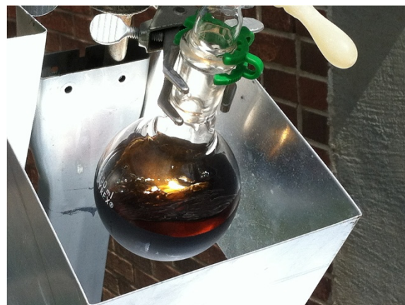
Figure 2 Close up view of painted flask. Round bottom flasks were painted black half-way up the flask using VHT® Flame Proof paint, which can withstand intermittent temperatures up to 1093°C. The round bottom flasks were painted black in order to prevent photochemical side reactions and to allow for a more efficient heating process.
