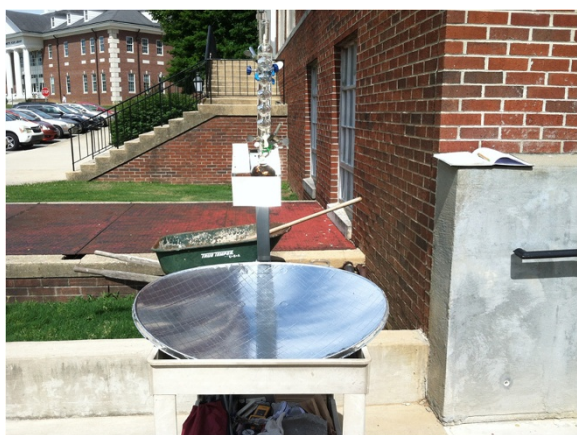
Figure 1 Solar reflector set-up. A solar reflector was designed through the repurposing of an unused satellite dishes into a reflective parabolic mirror that will serve as the sole heat source to drive synthetic chemical reactions to completion. Satellite dishes were completely covered with Metalized Mylar® tape to attain the reflective properties needed to generate heat.
