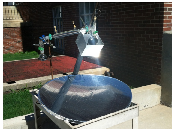
Figure 4 Solar distillation set-up. Distillation set-up to purify recovered glycerol.
