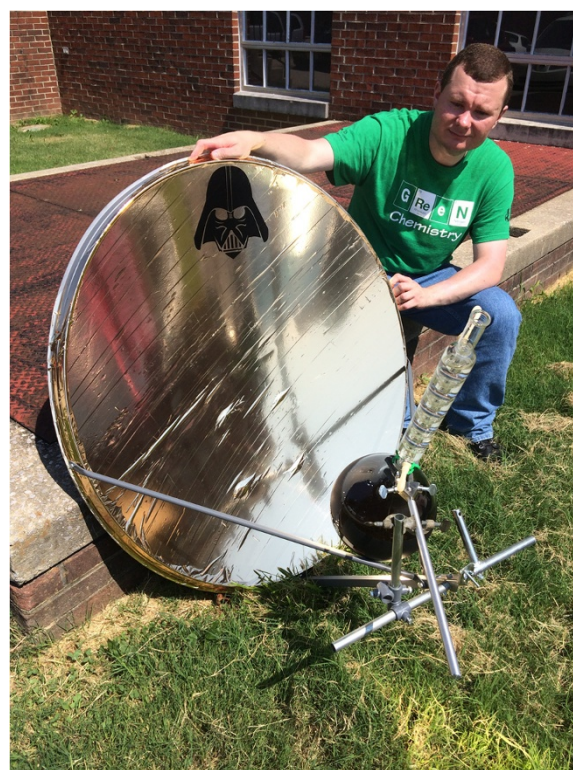
Figure 3 D.E.A.T.H dish set-up. Larger size dish to provide more surface area to expand procedure to larger scaled reactions.
