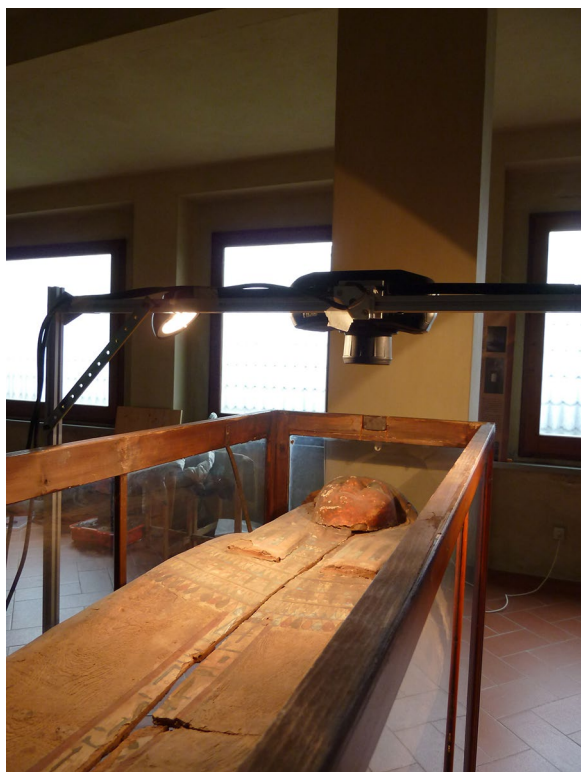
Fig. 2 The experimental set-up adopted to perform the in-situ measurements campaign on the Egyptian coffin: the HSI portable camera along with the illumination system on the bespoke mechanical structure
