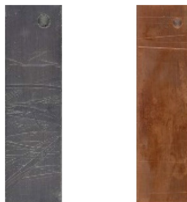
Fig. 3 Lead (left) and copper (right) coupons from Institution III previously abraded with glass brushes showing unsanded lines after testing materials 1 and 7, respectively
