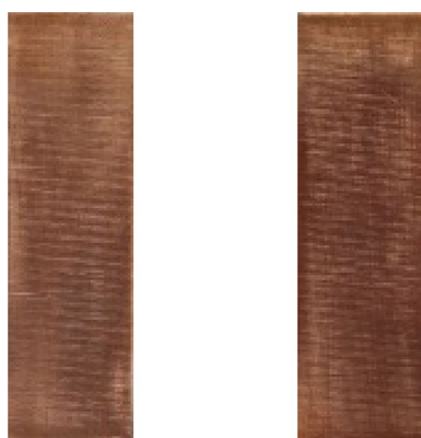
Fig. 2 Copper coupons from Institution VII abraded with 1800 micromesh pads showing horizontal unsanded lines after testing material 1 (left) and material 8 (right)
