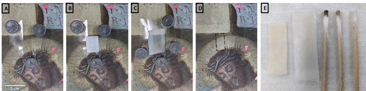
Fig. 10 Using the Nanorestore Gel® Peggy 6 for cleaning the sensitive brown; A Isolated the area to be cleaned and masked surroundings with Melinex™; B Placed pH 6.0 EDTA loaded Peggy Gel for 90 s and removed; C Placed pH 7.0 buffered rinsing solution loaded Peggy Gel for 60 s and removed; D Picked up the swollen crust with swabs; E The EDTA loaded Peggy Gel, the rinsing Peggy Gel and the swabs that picked up the crust
