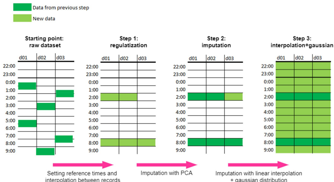
Fig. 5 Methodology followed for data reconstruction. Step 1: regularisation by means of interpolation, Step 2: Imputation of missing data, Step 3: Imputation with linear interpolation and Gaussian noise
