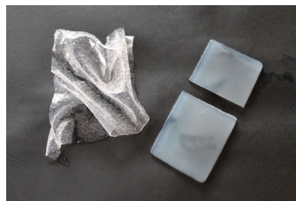
Fig. 6 Comparative image of the manipulable agar spray compared to the rigid agar obtained with traditional procedures
