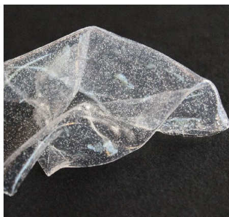
Fig. 7 Air bubbles incorporated in the thin gel layer
