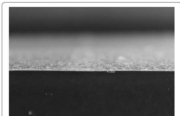
Fig. 5 The homogeneous and thin film of agar spray obtained after atomization
