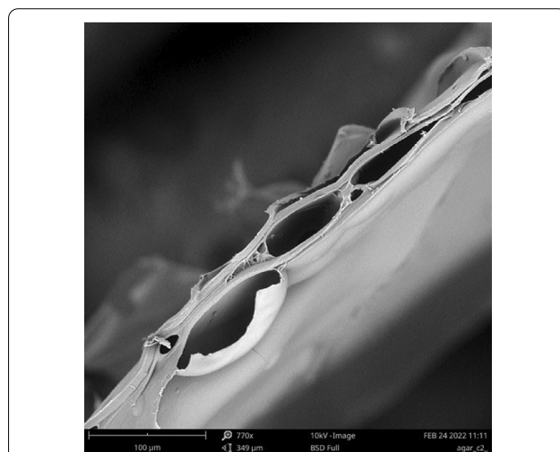
Fig. 11 SEM image of freeze-dried CTS spray agar at 3% w/v, polymeric foam structure
