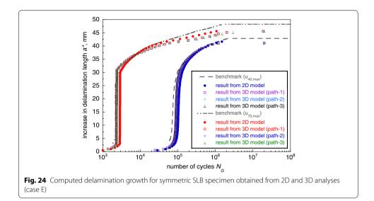
values to compute growth rates, da/dN, for intermediate mode ratios e.g.  $G_{II}/G_T = 0.43$  or for mode ratios that were constantly changing with delamination length. The analyses yielded results (open symbols) that are in excellent agreement with the benchmark and captured the threshold where growth is expected to stop. Also, the unstable path where static propagation is reached was correctly predicted (open blue squares).
