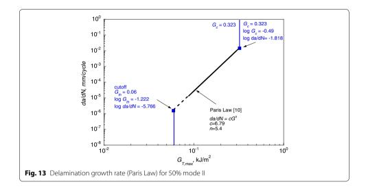
43% mode II as shown in Fig. 5) was obtained from the known growth relationship for 20% and 50% mode II shown in Figs. 12 and 13. The first step is to convert the known Paris Law data (Eq. 1) into log—log space such that
