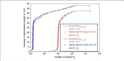
**Fig. 22** Computed fatigue delamination growth for symmetric SLB specimen (case D for  $u_{max} = 40\%$ , 70%  $u_c$ —ABAQUS tabular input for  $G_{II}/G_T = 0.2$  and 0.5)
