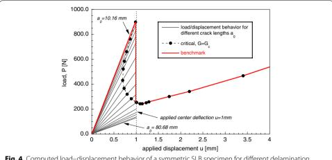
**Fig. 4** Computed load–displacement behavior of a symmetric SLB specimen for different delamination lengths  $a_0$ , calculated critical behavior and resulting benchmark case
