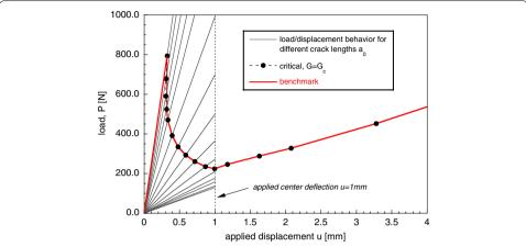
**Fig. 6** Computed load–displacement behavior of an unsymmetric SLB specimen for different delamination lengths,  $a_0$ , calculated critical behavior and resulting benchmark case
