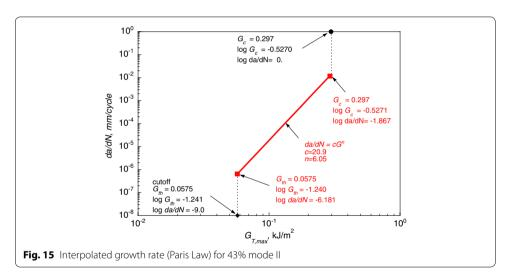
da/dN, for a target point (red circle) with any computed combination of  $G_T$  and mode ratio  $G_{II}/G_T$  can now be calculated. This scheme can easily be implemented into a spread sheet calculation or a software subroutine and was used to determine the Paris Laws for the symmetric (fixed 43% mode II) and unsymmetric (fixed 38% mode II) SLB specimen as shown in Figs. 15 and 16.
