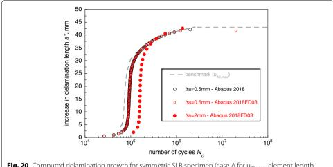
**Fig. 20** Computed delamination growth for symmetric SLB specimen (case A for  $u_{40,max}$  element length  $\Delta a = 0.5$  mm and  $\Delta a = 2$  mm)
