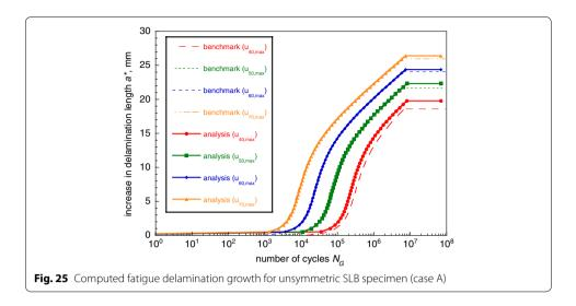
For all load levels, the results agree well with the benchmark solutions. For high number of cycles, growth stops and the last point on the curves was added manually to indicate the cutoff. This cutoff consistently occurred for longer crack lengths compared to the benchmark. More detailed investigation is necessary to find the source of this discrepancy.
