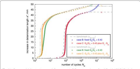
**Fig. 21** Computed delamination growth for symmetric SLB specimen (cases B and C with ABAQUS tabular input for fixed  $G_0/G_\tau$ = 0.43)
