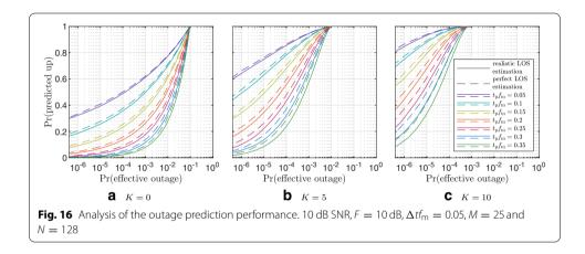
smaller. For higher prediction horizons  $t_p$ , the predicted channel coefficient has to be farther away from the origin to achieve the same outage probabilities. This is due to the fact that the variance of the error distribution is higher.
