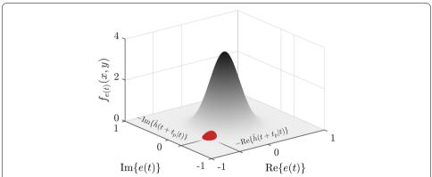
**Fig. 6** Illustration of the integration area to calculate the future outage probability. The red circle marks the integration area and has radius  $|h_{\min}|$
