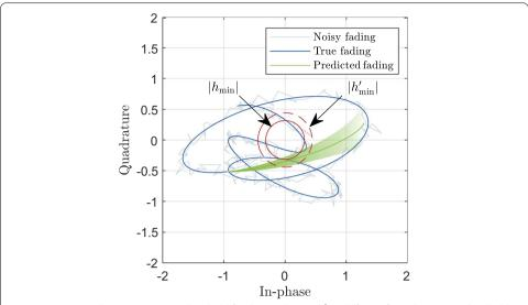
**Fig. 5** Outage prediction concept. A threshold for the prediction  $|h'_{min}|$  different from the outage threshold  $|h_{min}|$  is introduced to tune the prediction uncertainty
