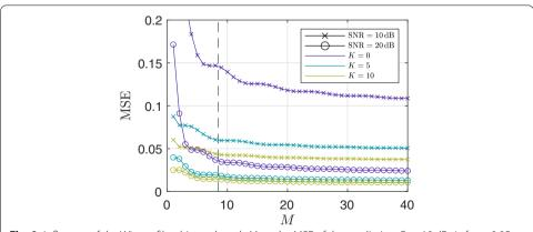
**Fig. 9** Influence of the Wiener filter history length M on the MSE of the prediction. F=10 dB,  $\Delta t f_{\rm m}=0.05$  and N=128; the dashed line is the point where  $M\Delta t$  equals an empirical value for the coherence time [6]
