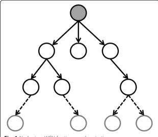
Fig. 1 Nodes in a WSN for time synchronization
