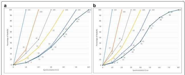
Fig. 6 Comparison of synchronization error when MBATS employs the designed path. a The densely deployed network case. b The sparsely deployed network case
