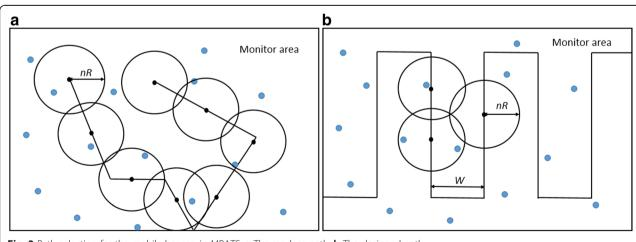
Fig. 3 Path selection for the mobile beacon in MBATS. a The random path. b The designed path
