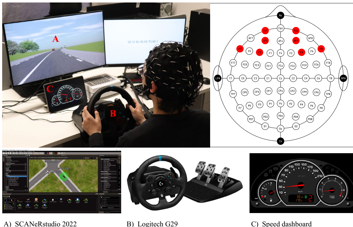
Fig. 1 Experimental simulation system
