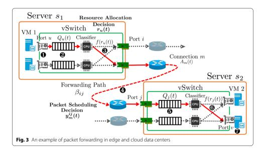
packets.  $\ref{vmu}$  VM2 receives packets of the connection  $\ref{m}$  from vswitch port  $\ref{vmu}$ , and handles the cognition service request. The cognition service response also can be presented as a similar process. Without loss of generality, we model all bidirectional service requests and responses as two connections (Table 1).
