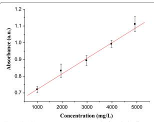
**Fig. 4** Absorbance versus concentration graph of standard caffeine in DMF
