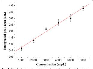
**Fig. 2** Graph of concentration versus integrated peak area for standard caffeine in water
