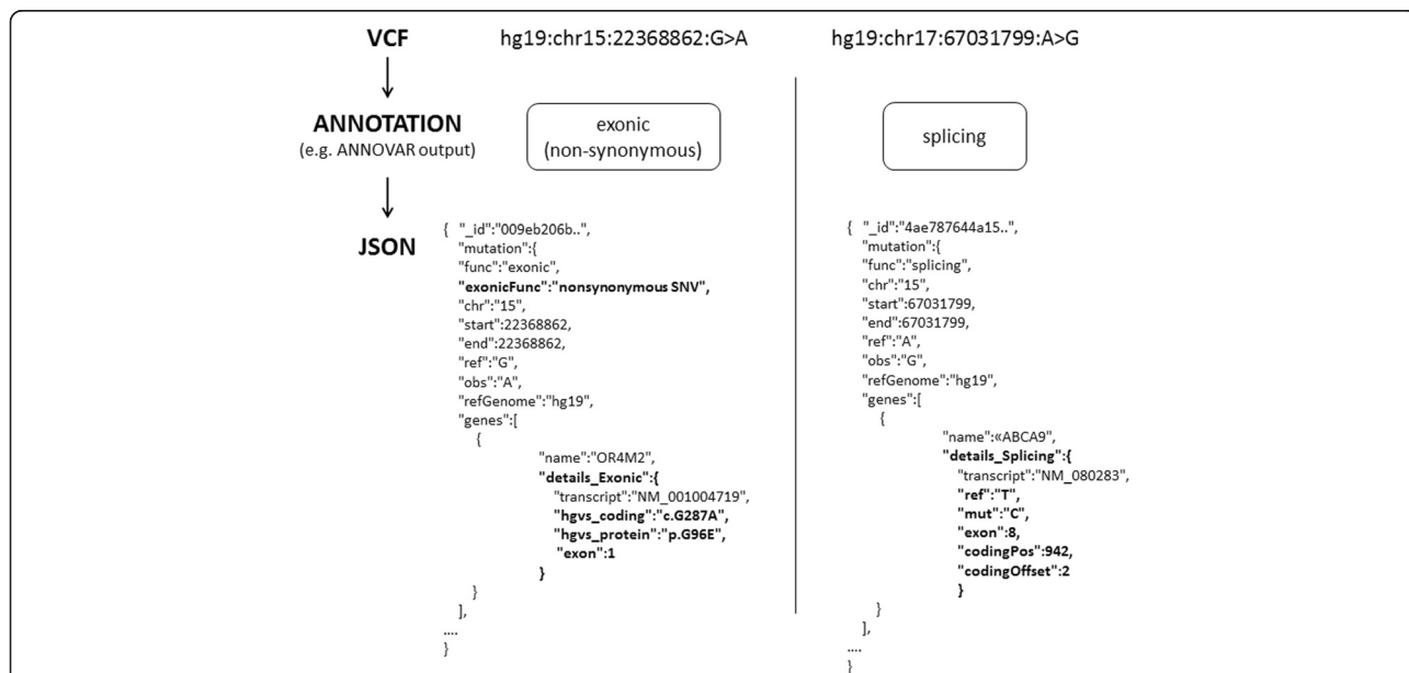
Fig. 2 Example of annotated variants in JSON format. Two variants, represented in VCF format, are identified by standard attributes (reference genome, chromosome, variant position and nucleotide changes). The annotation step finds out that one variant falls in an exon causing an amino acid substitution at the protein level (non-synonymous) while the other is located in a transcript splicing site. The two variants generate two different JSON objects, characterized by different attributes. Differences between JSONs are highlighted in bold
