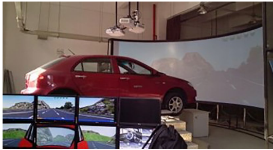
Figure 6 Hardware-in-the-loop simulation platform
