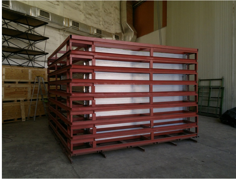
Figure 2 A picture of super blocks. A picture of the whole detector divided into eight super blocks (SBs). One SB is composed of 1/8 SciCRT supported by the steel-based structure to prevent the scintillator bars from deflecting by gravity.
