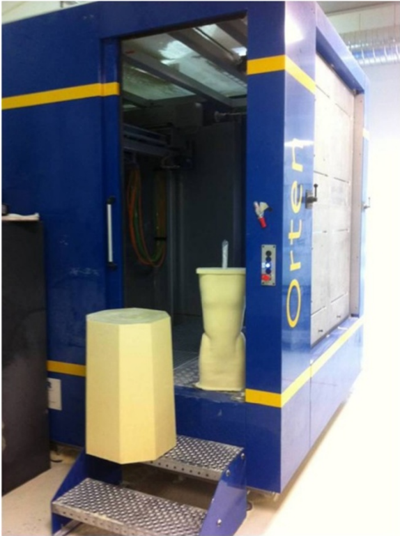
Figure 11 Milling different steps in rectifying positive.
