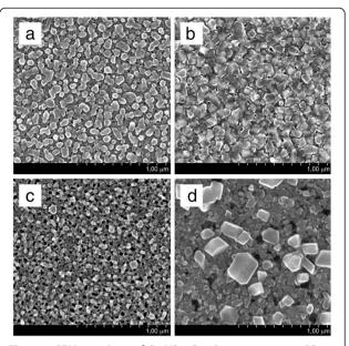
**Figure 2 SEM top views of Cu NPs.** Cu NPs were grown on PS with a thickness of 1  $\mu$ m and porosity of 50% to 55% (**a**, **b**) and 80% to 85% (**c**, **d**) by displacement deposition for 4 s (**a**, **c**) and 180 s (**b**, **d**).
