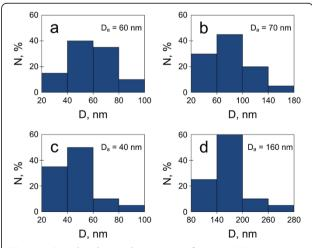
**Figure 3 Size distribution histograms of copper NPs.** Histograms were calculated for Cu NPs grown on PS with a thickness of 1  $\mu$ m and porosity of 50% to 55% (**a, b**) and 80% to 85% (**c, d**) by displacement deposition for 4 s (**a, c**) and 180 s (**b, d**).
