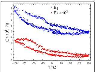
**Figure 10 Temperature variation of the Young modulus.** It was measured parallel to the pores or perpendicularly.
