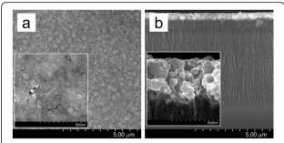
Figure 4 Top (a) and cross-sectional (b) SEM views of quasi-continuous Cu film. Cu film was grown on PS3 of 7- $\mu$ m thickness and 80% to 85% porosity by displacement deposition for 1020 s.
