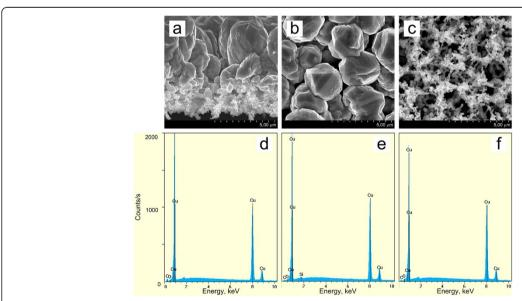
**Figure 8 SEM (a, b, c) and EDX point analyses (d, e, f) of the porous copper membrane.** The porous copper membrane was formed by displacement deposition of copper on PS4 for 7200 s from the solution of improved wettability; porous copper membrane was analyzed in cross section (**a, d**), top (**b, e**), and bottom (**c, f**).
