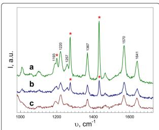
**Figure 11 SERS spectra.** (a) SERS spectrum of 10<sup>-6</sup> M CuTMpyP4 adsorbed on the top side of porous copper membrane. (b, c) Raman spectra of 10<sup>-6</sup> M CuTMpyP4 deposited from water and solution on bottom side of Cu membrane and porous silicon substrate, respectively. Laser plasma bands are marked by asterisks. Excitation wavelength was 441.6 nm.
