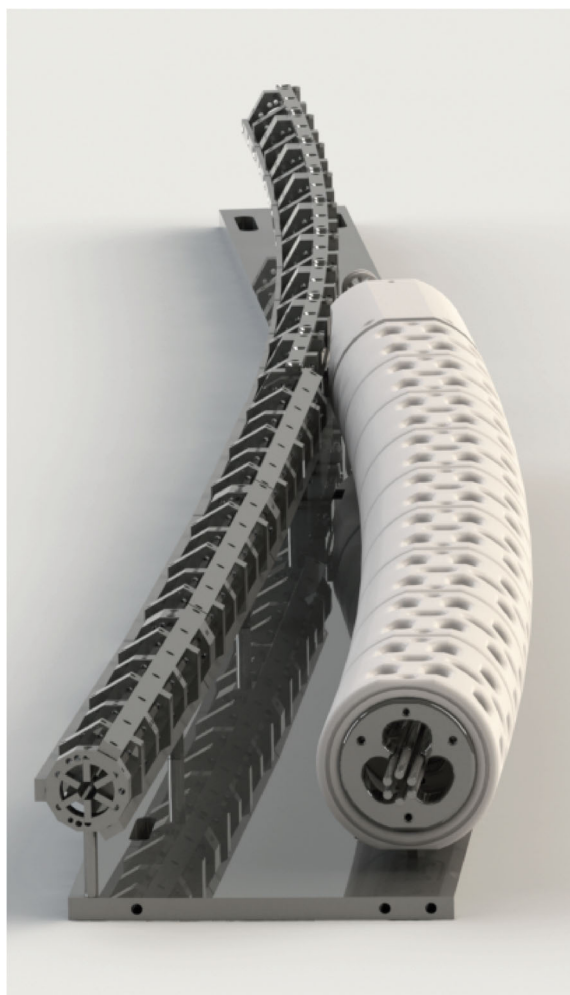
Fig. 6 Rendering of the two guides as used here. The left side shows the magnetic guide and the right side shows the electric guide
