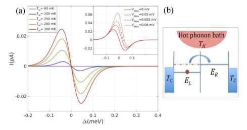
Fig. 3. (a) Zero-bias current as a function of  $\Delta$ , the difference between the energy levels of the dots, for different phonon temperatures. Inset: current as a function of  $\Delta$  for different biases and  $T_H=300\,\mathrm{mK}$ . Further parameter:  $T_C=60\,\mathrm{mK},~\Omega=0.05\,\mathrm{meV},~\Gamma_L=\Gamma_R=90\,\mathrm{neV}$ . (b) A sketch of a double dot system coupled to non-equilibrium phonon bath.
