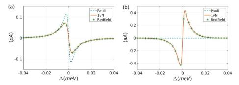
Fig. 4. (a) Zero-bias current as a function of  $\Delta$ , the difference between the energy levels of the dots, for Pauli, Redfield and 1vN approaches.  $T_C = 60 \,\mathrm{mK}, T_H = 300 \,\mathrm{mK},$   $\Omega = 0.001 \,\mathrm{meV}, \ \Gamma_L = \Gamma_R = 0.005 \,\mathrm{meV}.$  (b) Zero-bias current as a function of  $\Delta$ ,  $T_C = T_H = 60 \,\mathrm{mK}$ , other parameters are the same as (a).
