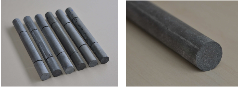
Fig. 4. UHPC specimens fractured in the spalling tests (left) and a typical fracture surface (right).
