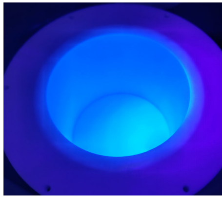
Fig. 14 ~ 3.0 m TPB has been coated on the inner wall of a 10-cm PTFE detector (top view)
