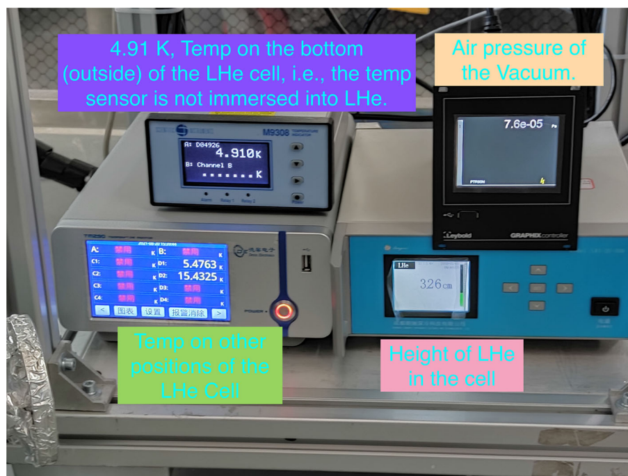
Fig. 5 The screen on the upper left shows the temperature on the bottom side of the 30 g detector (The temperature sensor did not immerse into the LHe.), so it is slightly higher than 4.5 K; however, the screen on the lower right clearly shows the height of LHe in the cell is 3.26 cm. The upper right screen is the vacuum inside of the stainless vacuum vessel. The lower left screen shows the temperature on the top side of the 30 g cell (5.4763 K) and the helium gas in the copper vessel (15.4325 K), respectively
