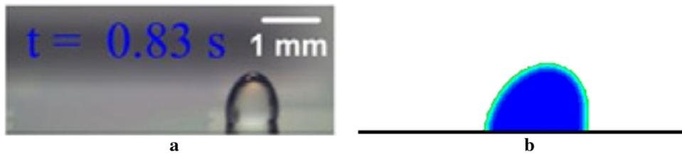
**Fig. 9** Droplet shape in pumping mode: **a** experimental data presented by Wang et al. [49] and **b** numerical results
