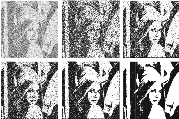
Fig. 8 Results by the proposed method and four traditional denoising methods. From left to right, the first line are the noisy image with GWN ( \mu = 0.5, \sigma = 1 ), geometric mean filtering and arithmetic mean filtering. The second line is the median filtering, Wiener filtering and the result of the proposed method
