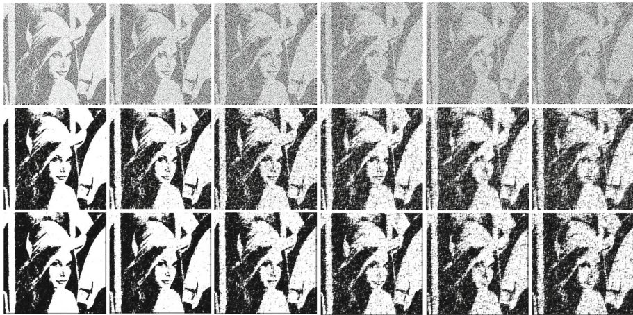
Fig. 7 Denoising results of the same image with different GWN parameters by either using the adaptive BSR method or the adaptive PSR method. From top to bottom, we show in the first row, the figures of the noisy images, in the second row, the results of the adaptive BSR, and in the third row, the results of the adaptive PSR. The variances of GWN added in the images are 0.5, 1, 1.5, 2, 2.5 and 3, respectively, while the mean is 0.5 in all cases
