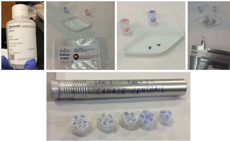
Fig. 2 Top: materials used to prepare the samples to be irradiated. From left to right: a liquid standard with certified concentration of trace elements, high-purity metal foils cut in small squares to fit into the PET vials, fragments of Ge crystal, Al–Co wires cut and shaped as small rings. Bottom: the PET vials packed to fit into the aluminum holder used for irradiations in the TRIGA-RC1 Central Channel
