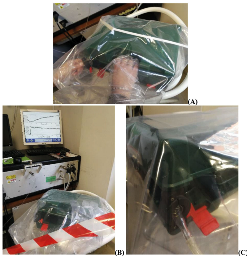
Fig. 4. An example of analysis using the cavity ring down laser spectroscopy technique: (A) put the sniffer of the spectrometer into the bag; (B) the analysis start; (C) detail of the sniffer into the bag.
