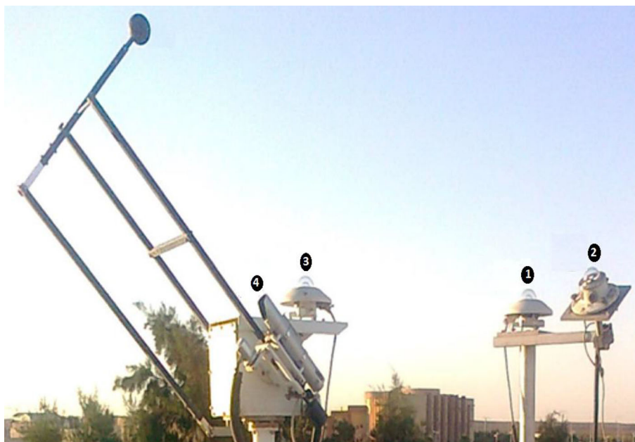
Fig. 3. Radiometric station: (1) Pyranometer for global solar radiation measurement on horizontal surface; (2) pyranometer for global solar radiation measurement on inclined surface; (3) pyranometer for diffuse solar radiation measurement on horizontal surface; (4) peryheliometer for DNI measurement.
