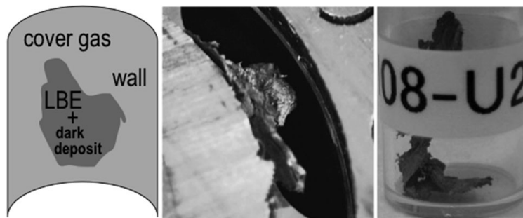
Fig. 5. Sampling of an LBE/cover gas-interface sample, H08-U2 that was sticking to the wall. Left: schematic view; middle: sample, H08-U2, sticking to the wall; right: the final sample. Figure reproduced from [6].
