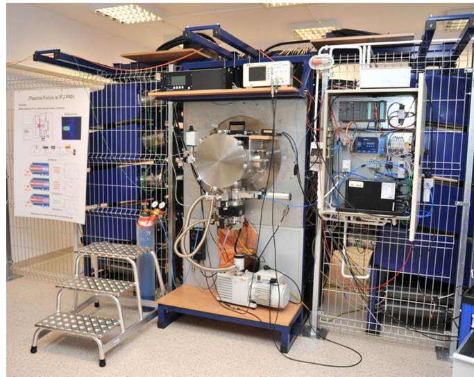
Fig. 1. Plasma focus (PF-24) device at IFJ PAN (Poland).
