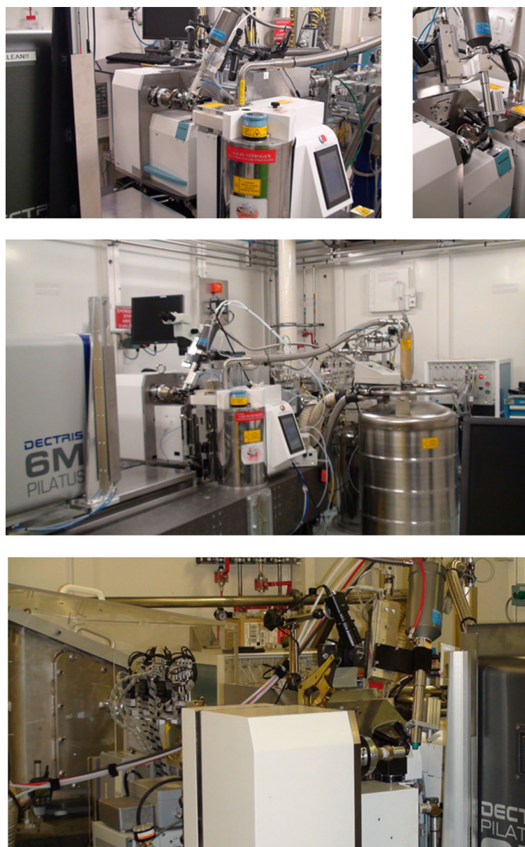
Fig. 3. The sample environment of ID29 (top) comprises a micro-diffractometer with mini-kappa goniometer mounted, a SC3 sample mounting robot, a fast-readout pixel array detector, a Cryostream 700 series cryocooler with annealing blade and a fluorescence detector. The sample environments of ID23-1 (middle) and ID23-2 (bottom) comprise the same elements based around a mini-diffractometer.
