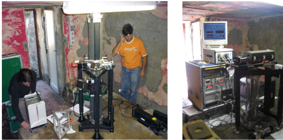
Fig. 3. Gravity station at Serra La Nave (SLN, Mt. Etna): on the left the FG5#238, on the right the IMGC-02 during the measurements.
