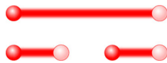
Fig. 164 The QCD string extends between a pair of test quark and antiquark (upper figure). The string breaking occurs once the fluxtube energy exceeds the meson mass (lower figure)
