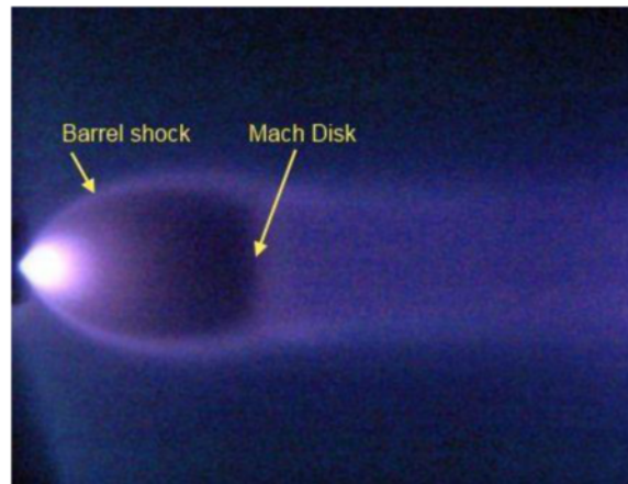
Fig. 1 CW gas jet expanding from sonic nozzle into poor vacuum (from [60]) showing the shock wave structure in jets. Barrel shock wave, Mach disk and the "Zone of silence [7]" between them are clearly visible in this rare photograph. The gas was made to glow by electron beam excitation
