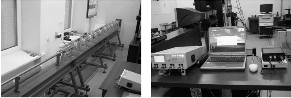
Fig. 1. General views of the Split Hopkinson Pressure Bar apparatus with data acquisition and control systems.
