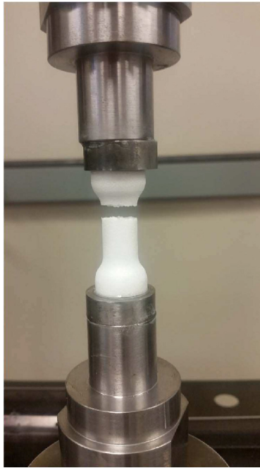
Fig. 4. Photograph of the tensile-test configuration and the failed tensile specimen.
