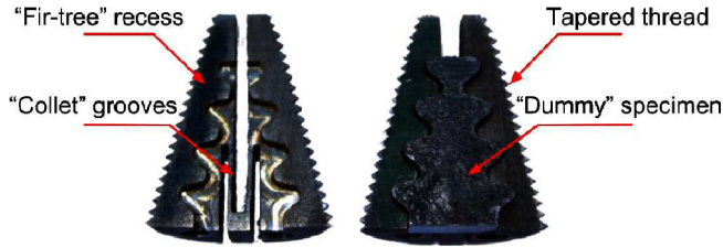
Fig. 2. The clamps used to secure the specimens in the Split Hopkinson Bar.
