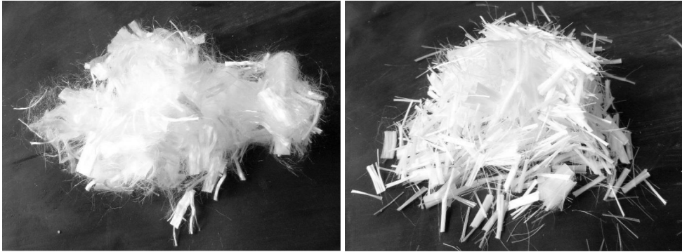
Fig. 1. The polypropylene (left) and polyvinylalcohol (right) fibres used.
